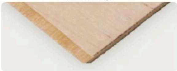
Veneer shortage in the inner layers
