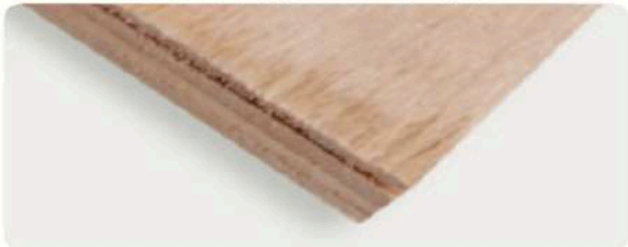
Veneer shortage in the inner layers
