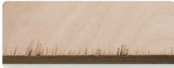
Shatters (defect due to cutting)
