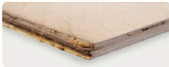
Shatters (defect due to cutting)
